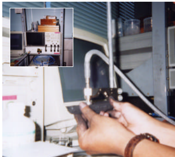
Figure 4.6. Measurement of burnt coal seam sample using dielectric constant kit HP85070B
